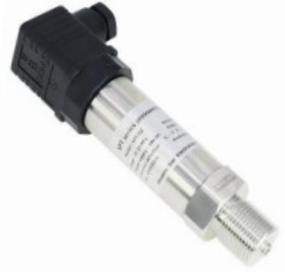
SP 21 Range: -1...0~0.1...1000bar Output: 4~20mADC Accuracy: \pm 0.5\% FS DIN43650 Connector
