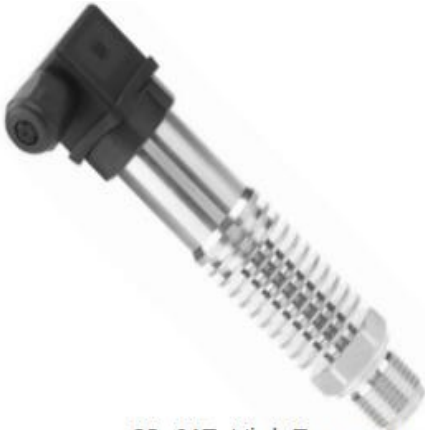
SP 21T High Temperature use Range: -1...0~0.01...1000bar Output: 4/20mA, 0/5V, RS485, etc Accuracy: \pm 0.5\% FS Temperature up to 250°C
