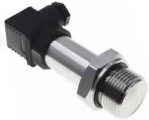
SP 21PC4 G1 flush diaphragm Range: -1...0~0.1...350bar Output: 4~20mADC, etc Accuracy: \pm 0.5\% FS DIN43650 Connector
