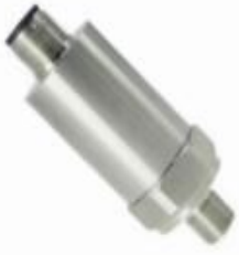
SP 21C1 Range: -1...0~0.1...200bar Output: 4~20mADC Accuracy: \pm 0.5\% FS M12x1 Connector
