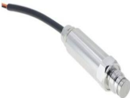
SP 21Y String Gauge Pressure Transmitter Range: 0~10...3000bar Output: 4/20mA, 0/5V, RS485, etc Accuracy: \pm 0.5\% FS
