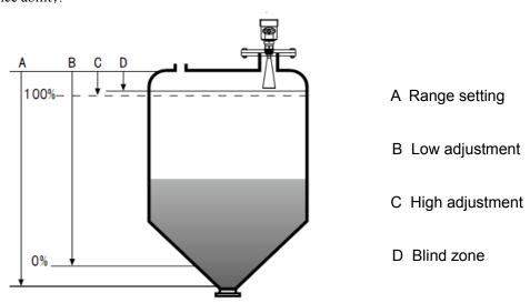
The reference plane for measurement is: the bottom surface of the thread or the sealing surface of the flange.
