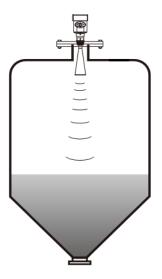
When there is a material pile, the antenna should be aligned perpendicular to the material surface. If the material
