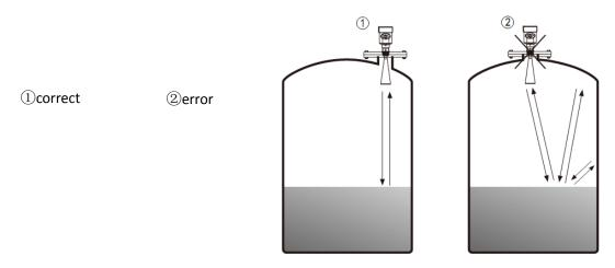
➤ When there are obstacles in the tank that affect the measurement, a reflector should be added to measure normally.
